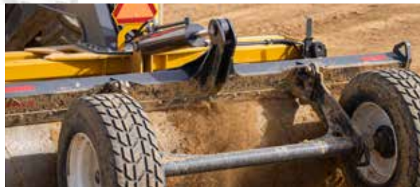
Mud scraper stops material buildup on drum
