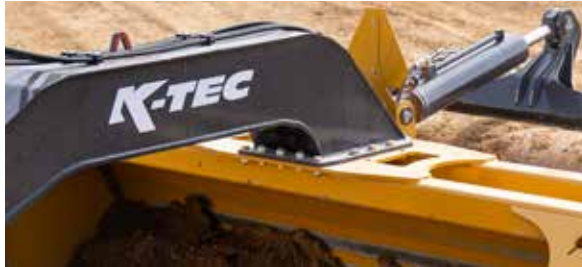
Bolt-on rotational hitch pole for transport of multiple units within width restrictions
