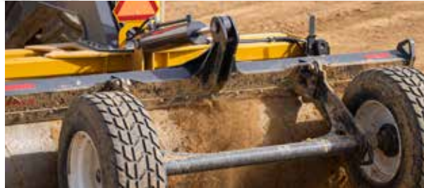
Mud scraper stops material buildup on drum
